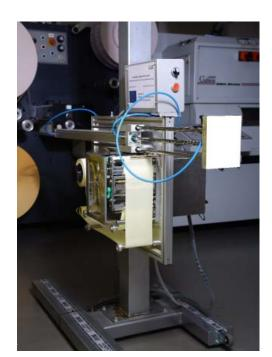
The entire process of identification can be effectively automated, indeed, from the object marking to the multiple readings. When it is necessary to apply a label on the item label additionally, we can use an automatic applicator with a telescopic arm instead of the usual manual application.
